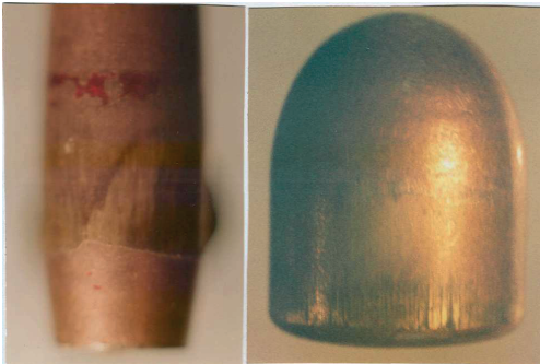
Photo 4. Traces on the surfaces of bullets fired from a smooth-bore craft-made firearm, exceeding the caliber of the barrel channel + 1.0 mm (on the left, bullet from a 5.45x39 cartridge, on the right, 9x18)
