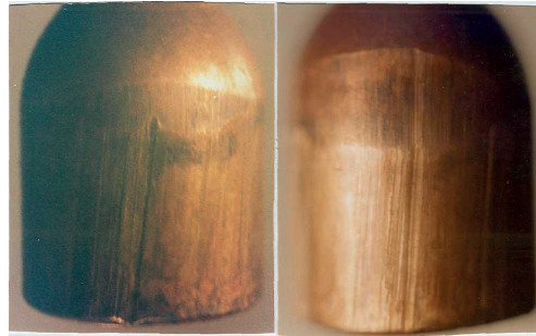
Photo 5. Traces on the surfaces of bullets that were reflected when fired from a craft-made firearm, in which the chamber (photo on the left) and the drum chamber (photo on the right) are misaligned
